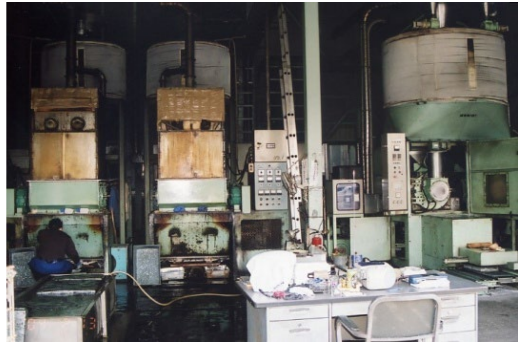
↑ Machines compressing EPS Fish Boxes at Tsukiji Fish Market in 2004. Photo by M. Kojima
